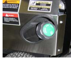
Fuel Tank: Corrosion proof polyethylene fuel tank
