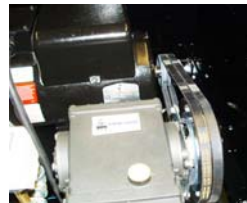
Pump-Saver Clutch System: Eliminates bypass overheating
