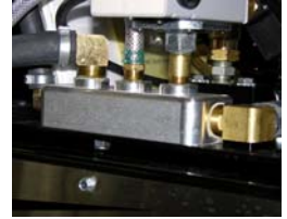
Manifold Assembly: Fewer connections and easier accessibility
