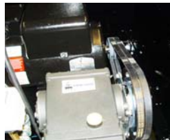
Pump-Saver Clutch System: Eliminates bypass overheating
