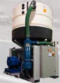
**The modular design requires only 25 ft<sup>2</sup> of space. Easy installation using a reclaim pit and almost any site configuration**
