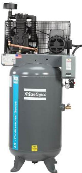
AR piston Compressors are splash lubricated, two-stage, aluminum compressors with a maximum operating pressure of 175 psi. All models are equipped with a magnetic starter as standard. Packaged models (\*PD) include a low oil level switch and pneumatic drain.
