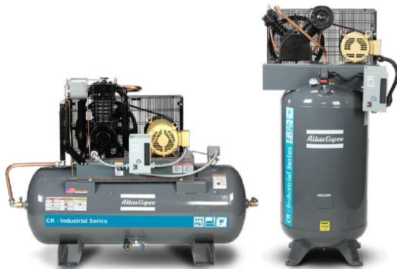
CR piston compressors include a cast-iron pump and are splash lubricated, two-stage compressors with a maximum operating pressure of 175 psi. All models feature a magnetic starter, electronic auto drain, low oil level switch, and belt guard-mounted after cooler.
