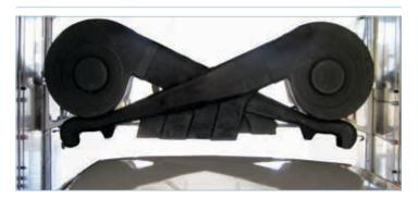
Contour-following dryer (shown) tracks vehicle from optimal distance to dry thoroughly while minimizing energy consumption and avoiding obstacles. Static onboard and freestanding dryers are also available.
