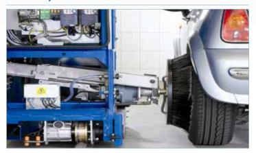
Our premium wheel cleaning system is angled for better centering, has larger brushes for better coverage, and integrates high pressure for added cleaning power. Our basic HubScrub® system is also available.
