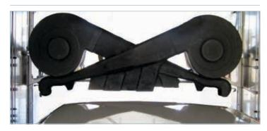
Contour-following dryer (shown) tracks vehicle from optimal distance to dry thoroughly while minimizing energy consumption and avoiding obstacles. Static onboard and freestanding dryers are also available.
