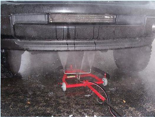
The Bottom Feeder V2TM utilizes a full stainless steel, 4 nozzle rotating assembly that covers approximately 24" of cleaning area.
