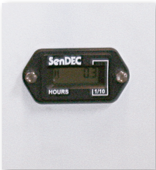
Hour meter displays the number of hours compressor has been in operation
