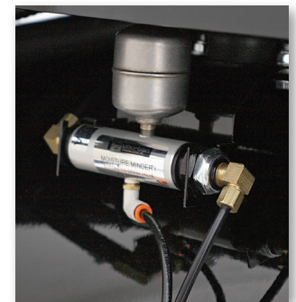
Tank drain automatically drains liquid from air receiver
