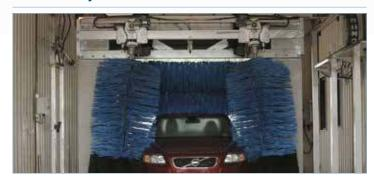
Side washers angle out on the first pass and in on the second pass, ensuring that curved surfaces at the top and bottom are thoroughly scrubbed.
