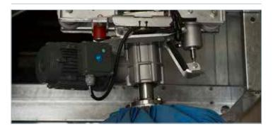
Electric rotation and drive motors eliminate risk of messy hydraulic leaks found in other systems that can disrupt operations and impact customer service.
