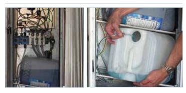
Chemicals are positioned inside the frame to eliminate the need for an equipment room or locating messy barrels inside the wash bay. Uses standard 5 gallon containers for easy handling.
