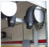
20hp and 30hp on-board dryers can be selected for shorter bays. For longer bays, 30hp and 40hp freestanding dryers can increase throughput by enabling the next car to load while the previous car is being dried.
