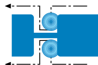
Adjustable draw bar limit for side brushes
