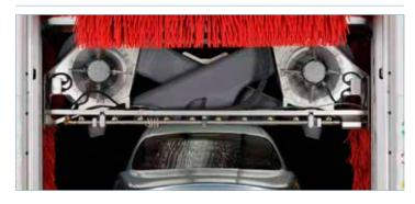
Tracks vehicle from the optimal distance to minimize energy consumption while avoiding obstacles such as antennas and roof racks. AquaDri® static on-board and freestanding dryers are also available for the ChoiceWash XT.
