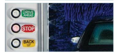
Bright green, red and yellow lights augmented by reflective decals on both sides of the gantry ensure customers are safely guided into position.
